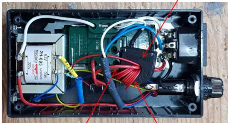
Current Transformer (CT)
